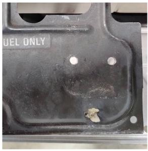
5. Place Plate Caddy over holes and pass one  $\frac{1}{4}$ -20 screw from license plate side towards the caddy thu the slotted holes.
