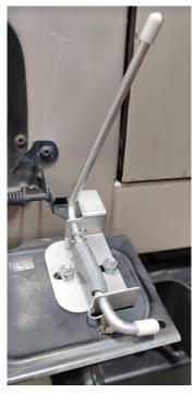
7. Rotate the long arm down to the left and flip up the license plate bracket to close it. Note where the short arm of the Plate Caddy comes into contact with the vehicle surface. Clean that location and place the provided 1"x1" adhesive backed protective film to that location.
