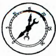
RESTRICTED EXHAUST (DROPS TOWARDS ZERO AS ENGINE RPM INCREASES)
