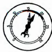
POOR VALVE SEATING AT IDLE
