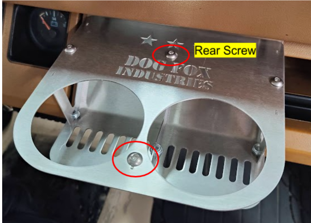
Figure 14. Install Rear Screw and Nut prior to Front Screw and Nut
