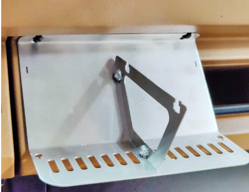
Figure 10. Base Plate with Center Support attached to dash
