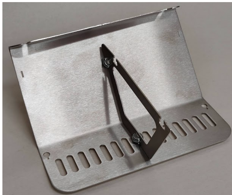
Figure 7. Center Support Fully Attached to Base Plate
