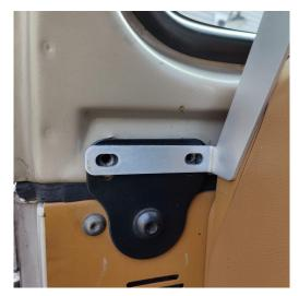
2. Place the mounting bracket against the windshield plate and thread both windshield bolts in by hand. It may help to use the T40 socket manually to get the bolts finger tight. The bracket should be slid up tight to the side of the dash.
