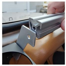
6. Using a ½-20 screw and washer, thread the screw into the center hole of the aluminum extrusion and finger tighten. Repeat on the opposite side
